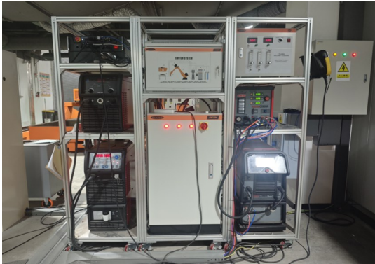
图1 等离子熔覆设备示意 Fig. 1 Schematic of plasma cladding equipment
