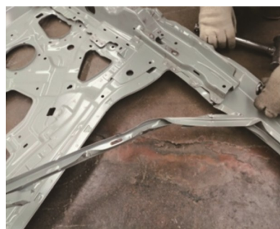
(b)门锁处焊点凿检
