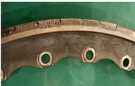
图 2 导向器内环端面磨损 Fig. 2 End-face wear of the guide vane inner ring
