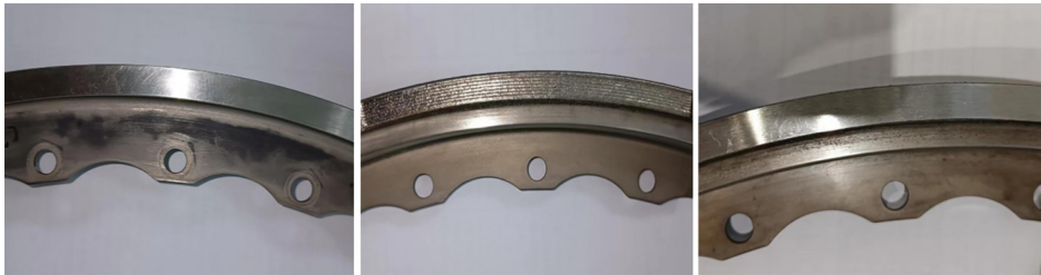
(a)去除涂层 (b)激光熔覆后 (c)表面磨加工后
