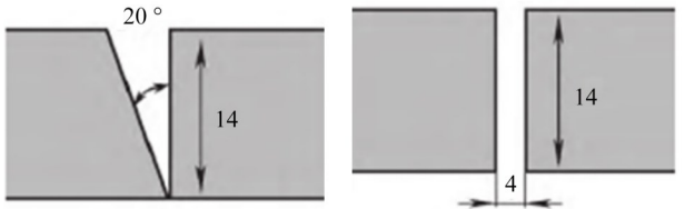
(a)单边V型坡口对接接头 (b)预留4 mm间隙的对接接头 图9 对接接头示意
