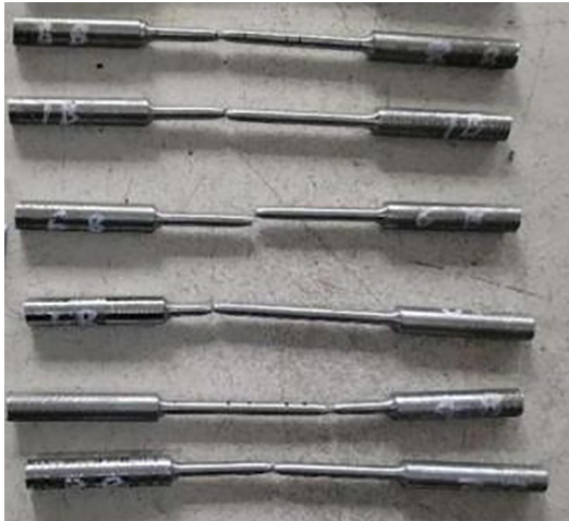
图3 40Cr 惯性摩擦焊接头拉伸断裂试样 Fig. 3 Fractured specimen of 40Cr inertia friction welded joints after tensile test
