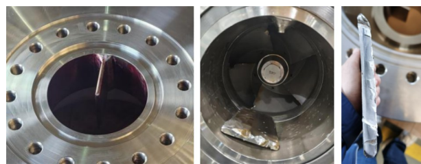
(a)初始完好状态 (b)整流板断裂后 (c)断口
